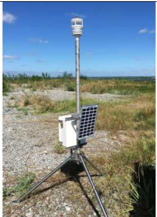
**Figure 3. Installed weather station**
