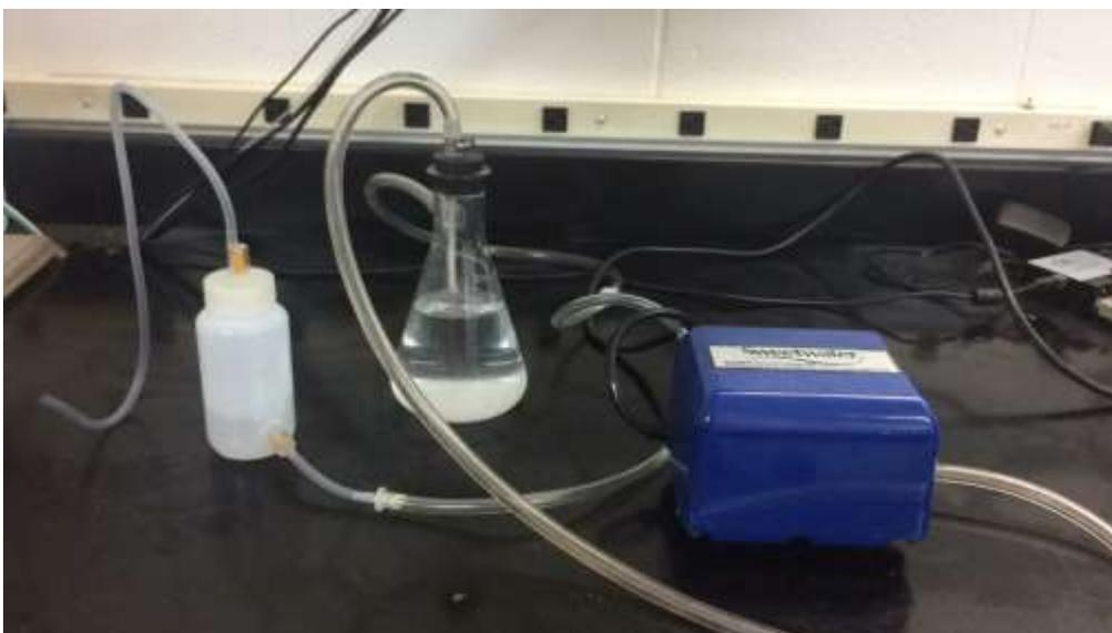
**Figure 3. Gas reactor prototype being tested using an air compressor and beaker of water for humidifying the air connected to the valve at the bottom of the chamber. Air successfully bubbled through the water at the bottom of the chamber and out the valve at the top of the chamber.**
