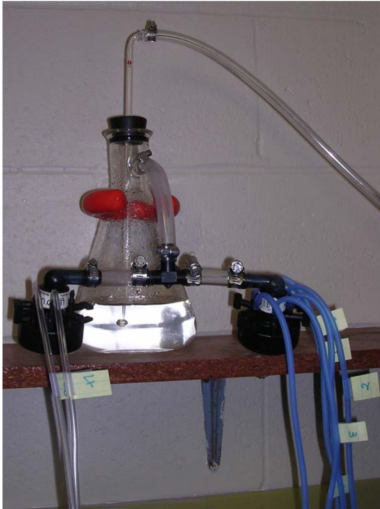
Figure 10: Upgraded aeration system.
