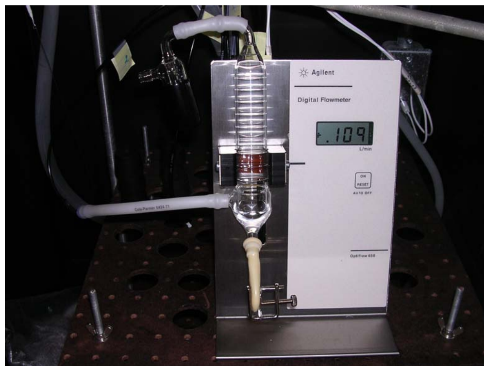
Figure 16: Measurement of the air flow rate.
