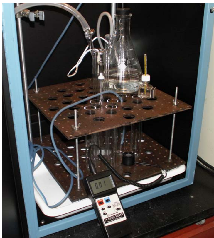
Figure 15: Checking the light sensitivity of the new PIMA photoreactor.
