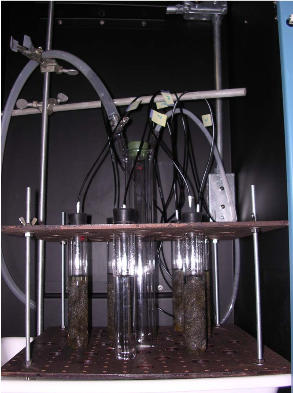
Figure 1: PIMA process reactor
