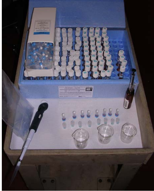
Figure 8: Preparation of the COD tests.
