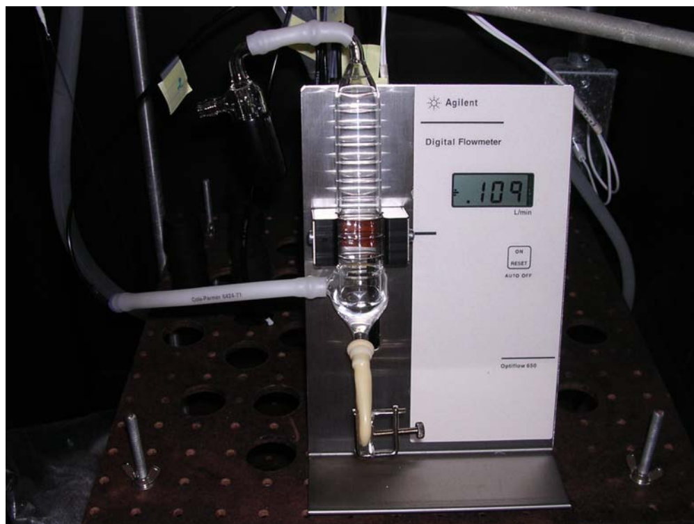
Figure 11: Measurement of the air flow rate.
