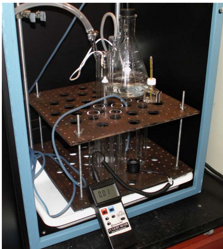
Figure 10: Checking the light sensitivity of the new PIMA photoreactor.
