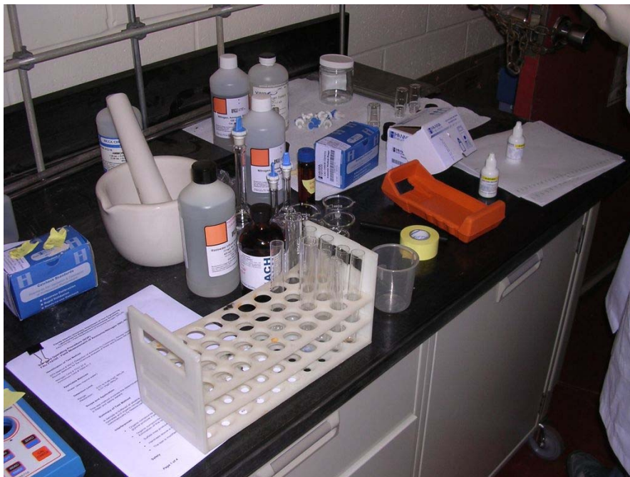
Figure 6: Laboratory bench scale ammonia analyses.
