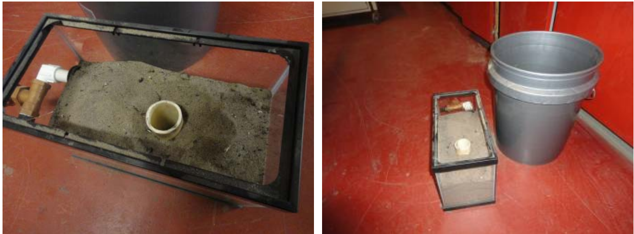
Figure 2. Construction of recirculating well installation
