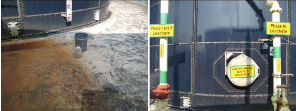
Figure 8. Leachate sample collection from Polk County facility.
