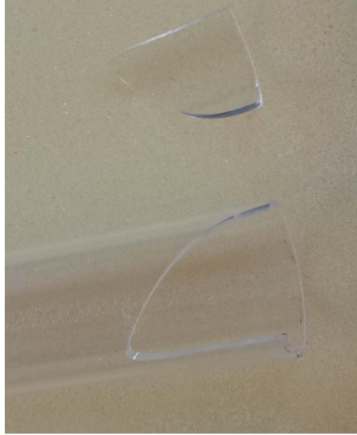
Figure 1: Broken Inner Lens
