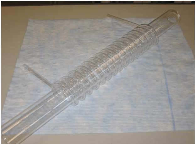
Figure 2. Custom quartz reactor coil
