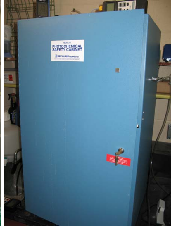
Figure 4. UV reactor safety cabinet
