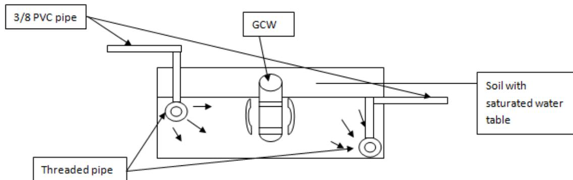
After balancing the flows, the three aquaria are going to be loaded from the same source of spiked water with different air flow rates to determine the optimum aeration rate to maximize iron removal and minimize plugging/fouling. The experimental setup is shown as follows:
