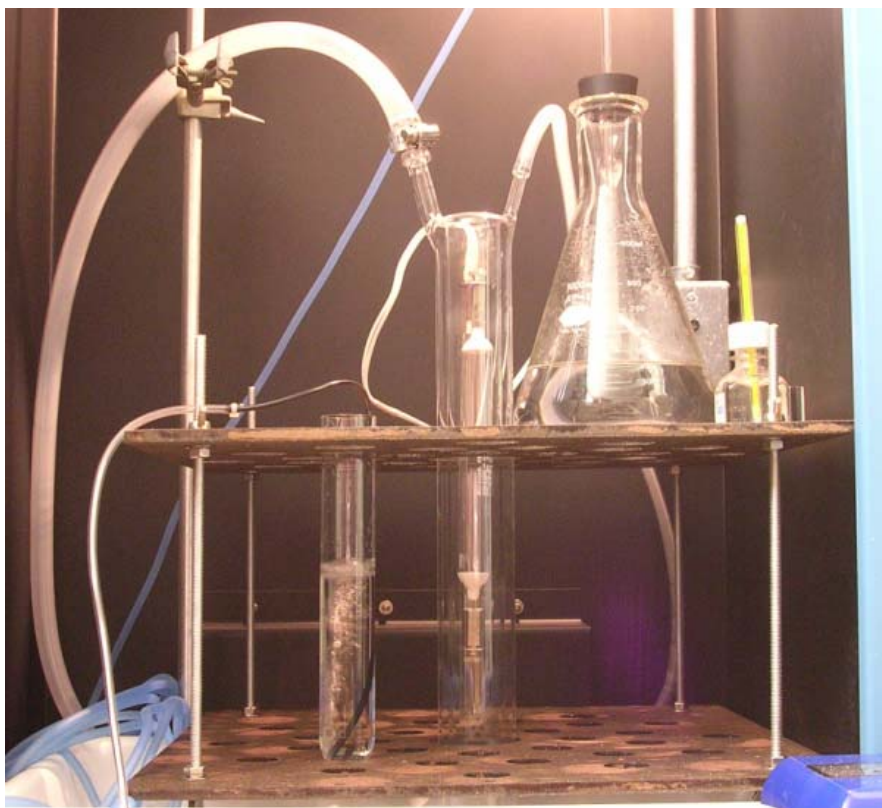
Figure 1: PIMA process reactor
