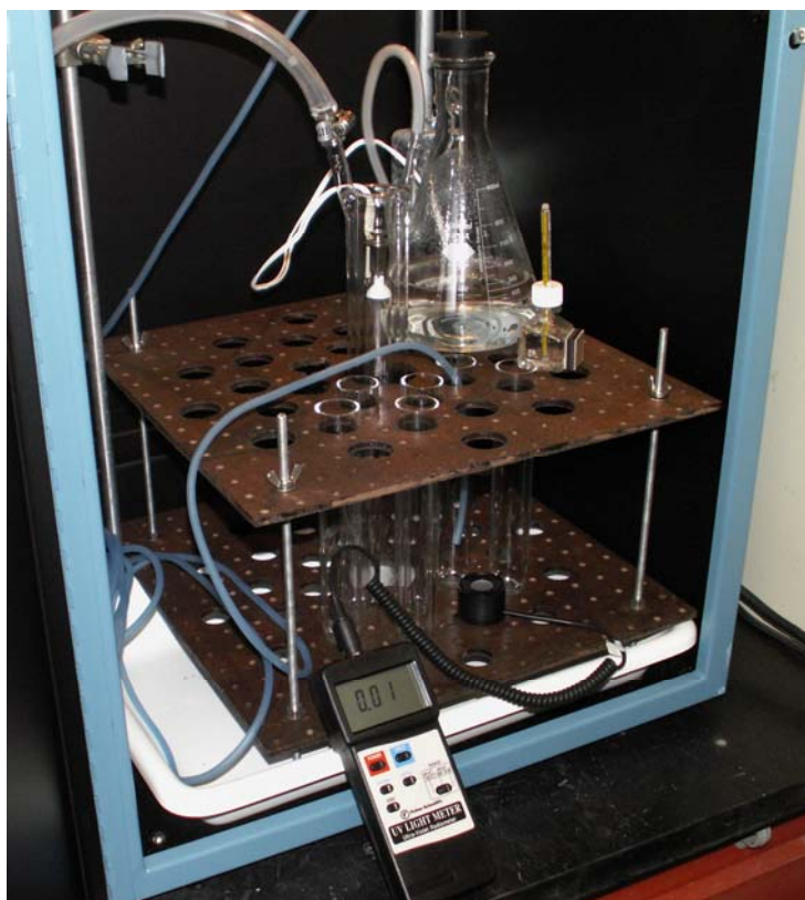
Figure 7: Checking the light sensitivity of the new photoreactor
