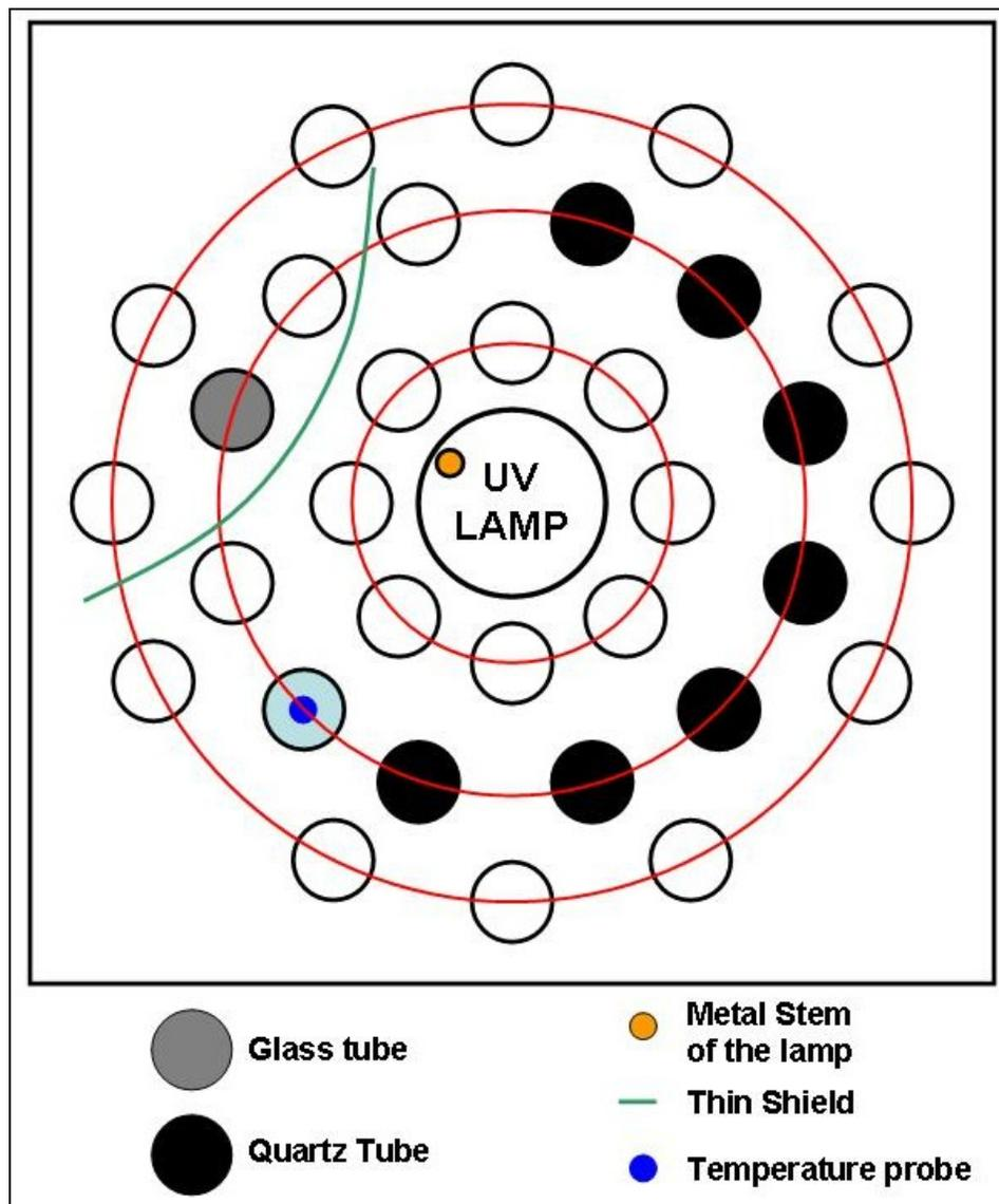
Figure 9: Reactor configuration with test tubes placement
