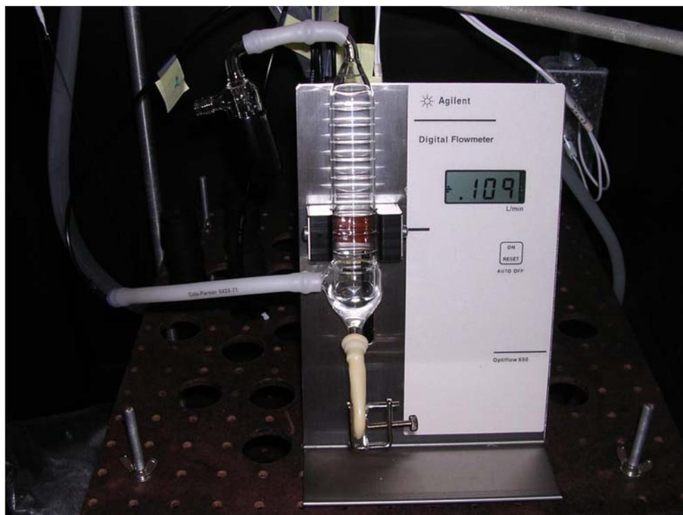
Figure 16: Measurement of the air flow rate.
