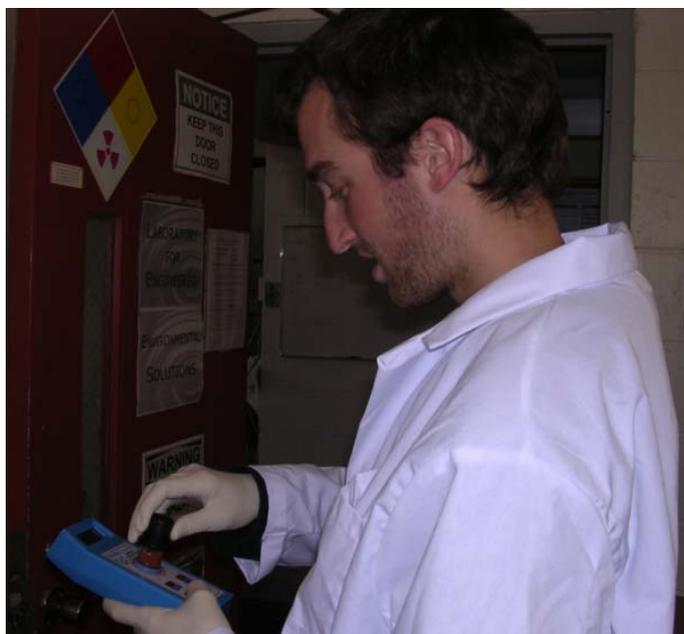
**Figure 2: Experiments to validate the ammonia meter.**
