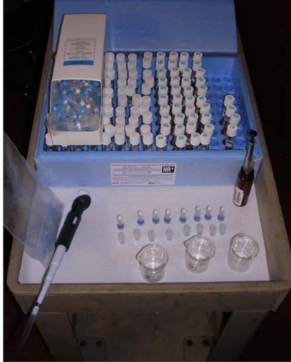
**Figure 13: Preparation of the COD tests.**
