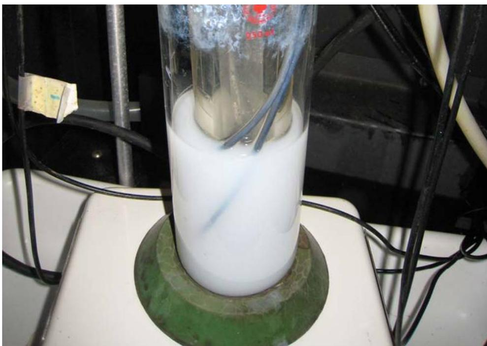
**Figure 22: Experiment #6 using an ammonia synthetic leachate with  $\text{TiO}_2$  particles (Degussa P25) at time,  $t = 5.0$  hours. Note no color change.**
