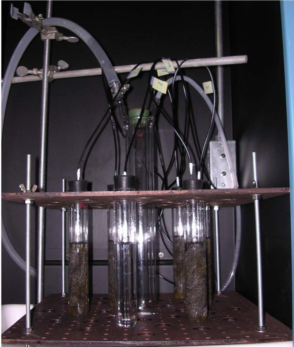
**Figure 1: PIMA process reactor**
