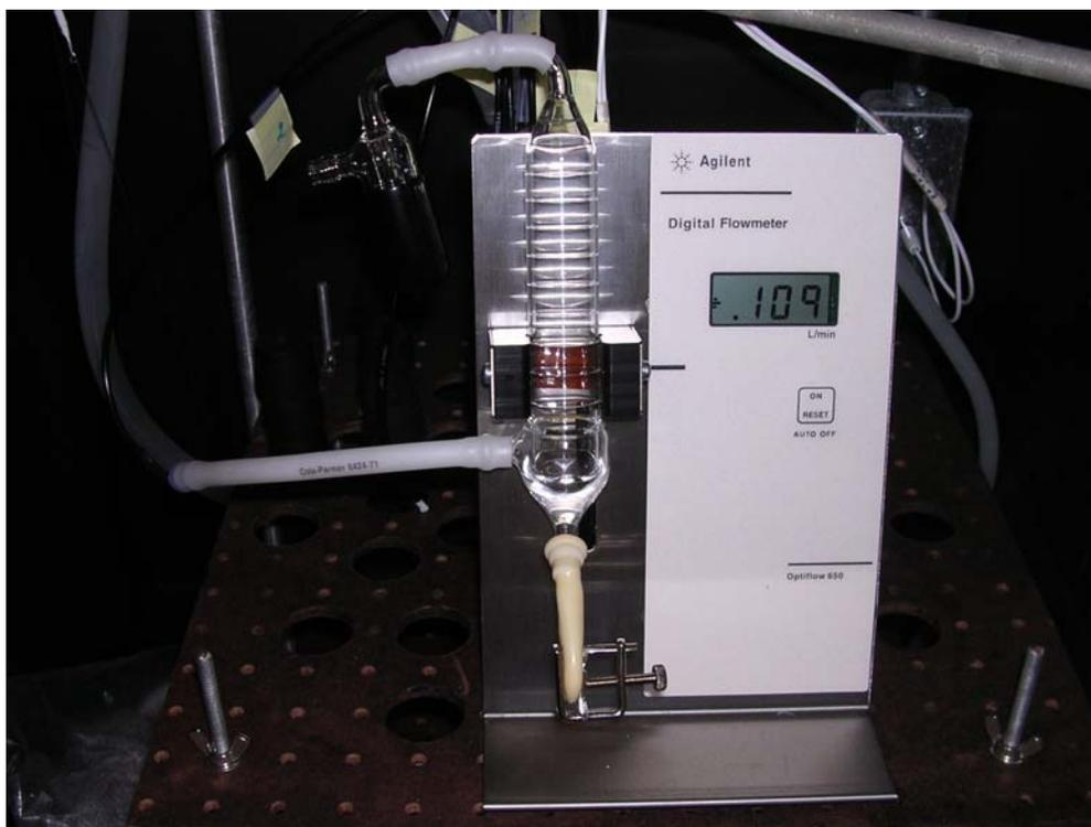
**Figure 18: Measurement of the air flow rate.**
