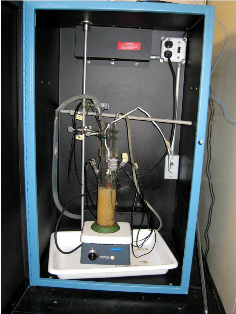
**Figure 2: TiO<sub>2</sub>-magnetite process reactor**
