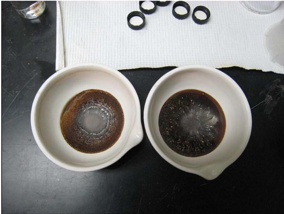
**Figure 23: Experiment #5: Reconditioning (drying at 105°C for 24 hours) of left over TiO<sub>2</sub> particles after treatment of synthetic leachate containing COD**
