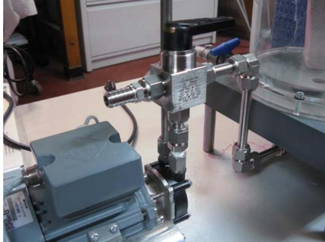
Figure 2. Three way valve modification for flushing and priming the recirculating pump.
