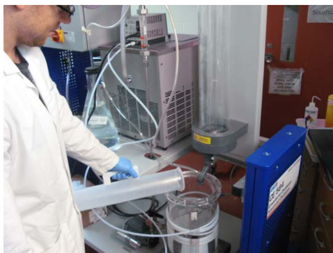
Figure 1. Frank Youngman testing the temperature control system provided by the recirculating chiller unit (in the background). The PTFE pipe is seen wrapped around the reaction chamber of the pilot unit in the foreground.
