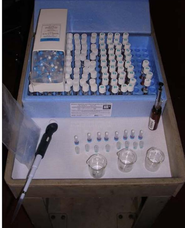
**Figure 7: Preparation of the COD tests.**
