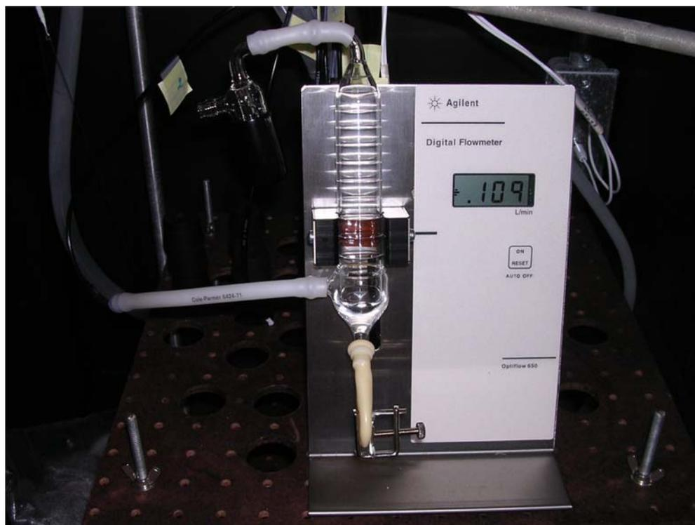
Figure 10: Measurement of the air flow rate.
