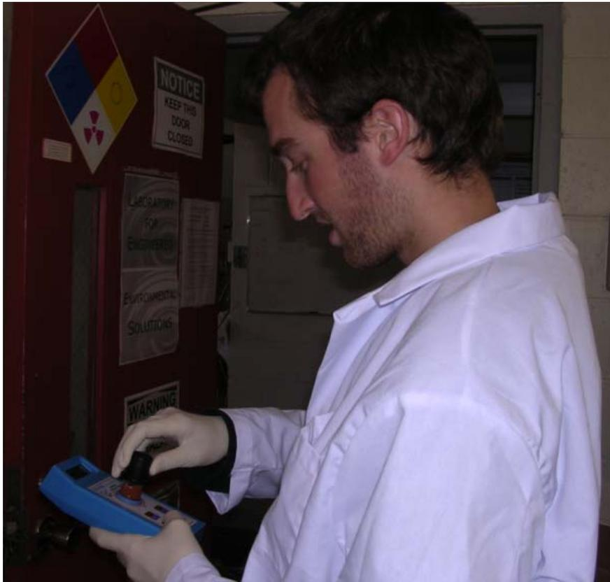
Figure 2: Experiments to validate the ammonia meter.
