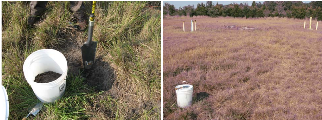
Figure 11. Soil sampling from the downstream SE corner (left) and from the upstream NE corner (right). The NE corner samples were taken just south of the monitoring wells that reported elevated iron readings.
