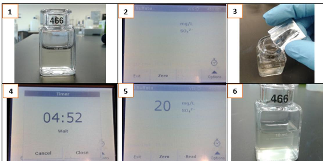
**Figure 34. Sulfate test flow path**
