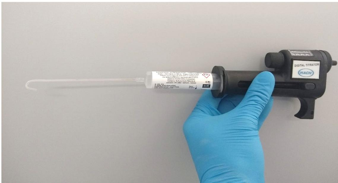
**Figure 23. Hach digital titrator setup for calcium measurement**
