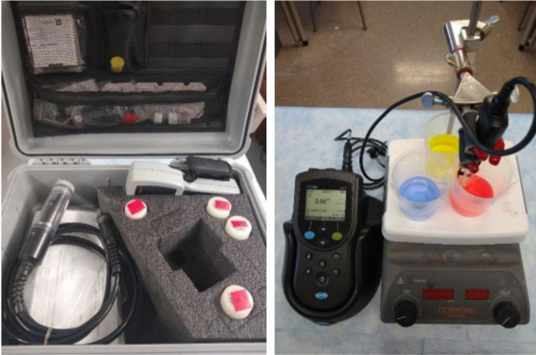
**Figure 21. pH measuring meters (YSI 556 MPS, left; Model Hq40d meter, right)**
