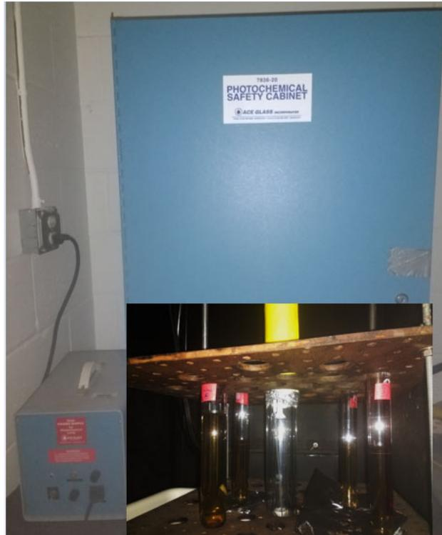
**Figure 15. Photocatalytic Safety Cabinet used to disinfect leachate in the laboratory**
