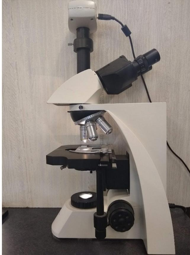
**Figure 28. Microscope with automatic camera (TCA-3.0) set up**
