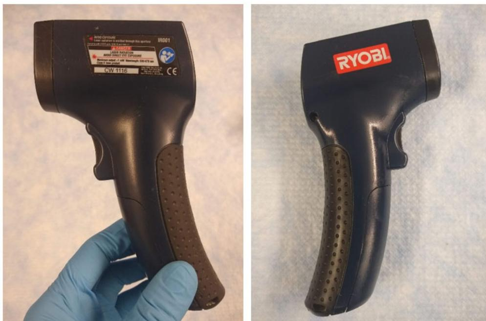
**Figure 22. Handheld thermal infrared thermometer (Ryobi IR001)**
