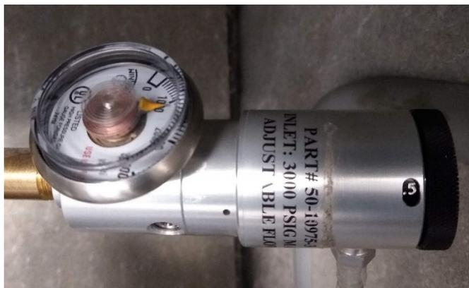
**Figure 17. Variable rate (0-3.5 lpm) gas regulator for 600 L gas cylinder**
