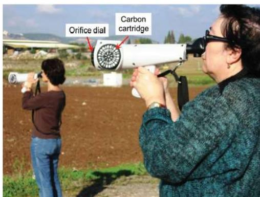
**Figure A6: Instruments used in field olfactometry (Laor et al. 2014)**
