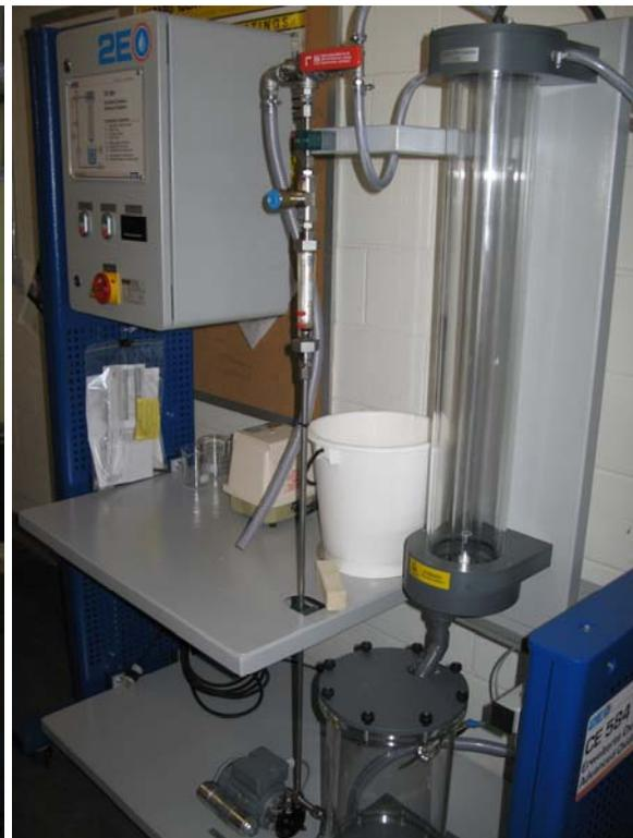
**Figure 6. Pump and treat pilot plant**
