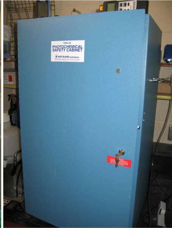
**Figure 4. UV reactor safety cabinet**
