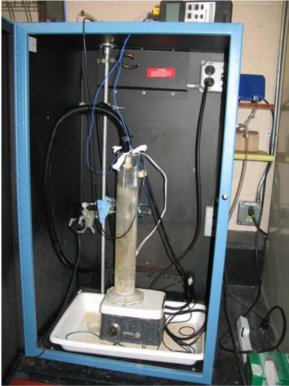
**Figure 3. UV reactor set-up**
