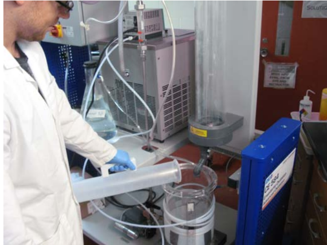
Figure 2. Frank Youngman testing the temperature control system provided by the recirculating chiller unit.
