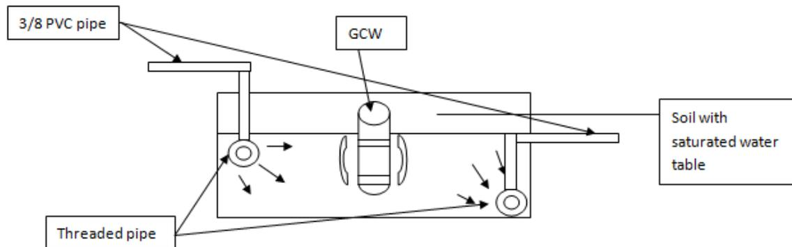
After balancing the flows, the three aquaria are going to be provided from the same source of spiked water with different air flow rates to determine the optimum aeration rate to maximize iron removal and minimize plugging/fouling. The experimental setup is shown as follows:
