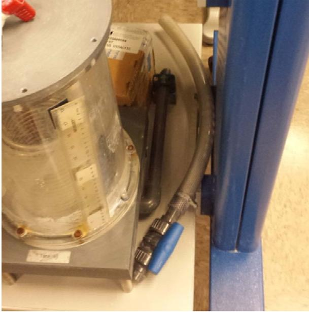
Figure 1: Broken Valve
