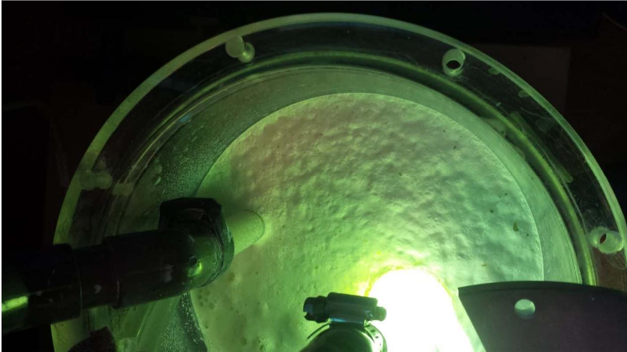
Figure 3: Foam in reservoir and flexible pipe to prevent foaming.
