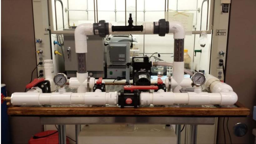
Figure 4: Critical Orifice Advanced Oxidation Device
