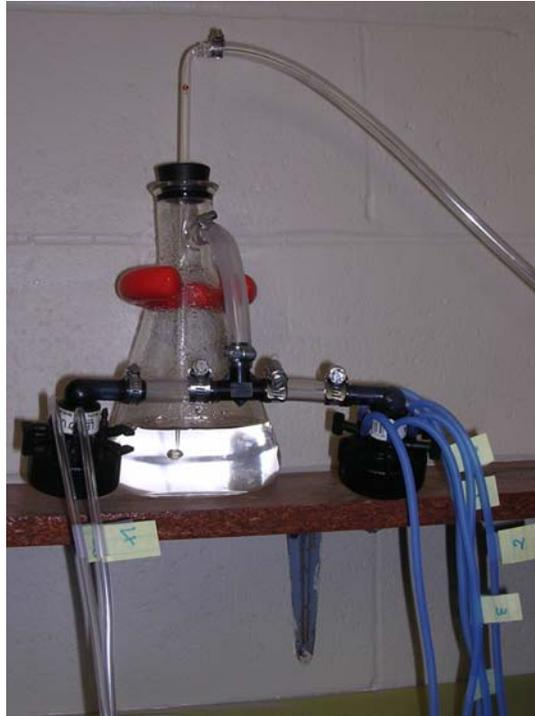
**Figure 2-3: Aeration and humidifier systems**
