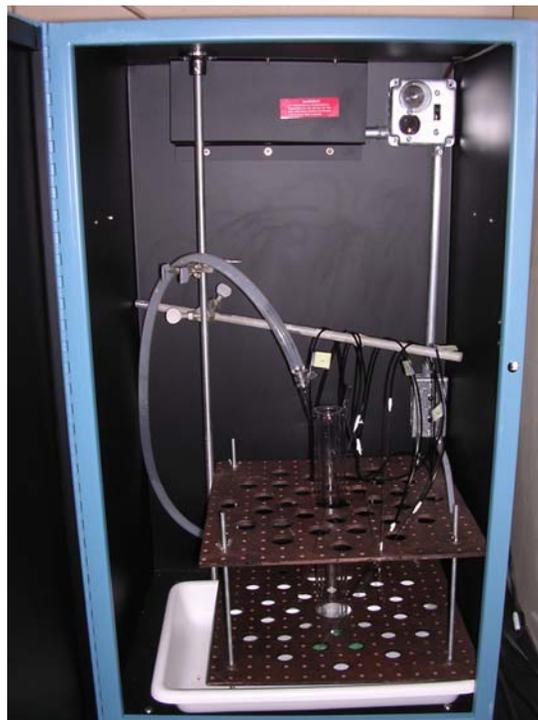
**Figure 2-4: View of the inside of the safety cabinet and aeration piping**
