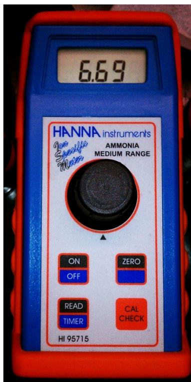
**Figure 29. Sample reading from HI 95715 Ammonia Medium Range ISM**
