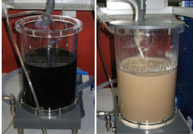
**Figure 62. Color comparison for raw leachate (left) vs. leachate w/ TiO<sub>2</sub> (right)**
