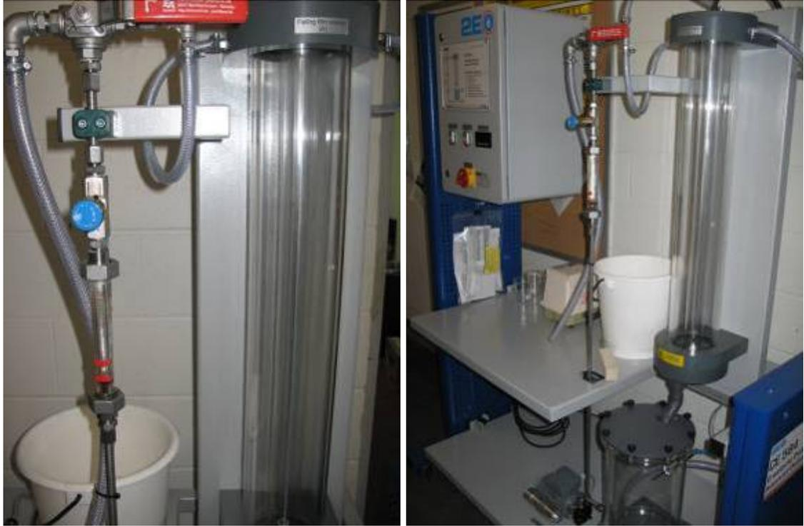
**Figure 10. Photographs of the falling film pilot reactor (left: close up view of the reaction chamber; right: overall view)**
