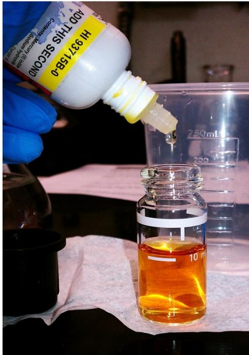
**Figure 28. Reagent addition to cuvette for ammonia testing**
