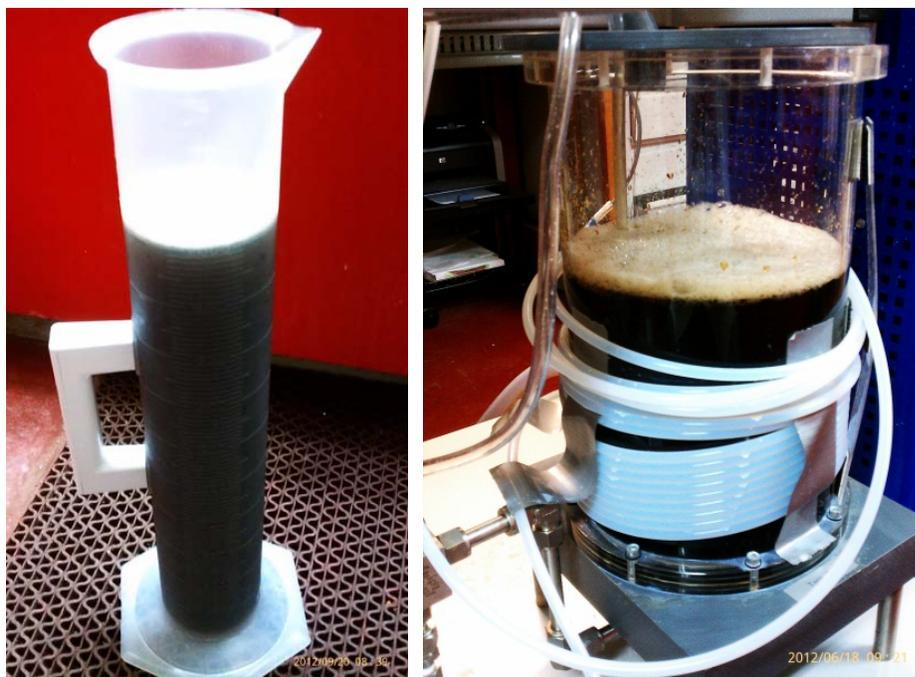
**Figure 23. Measurement of 2L of leachate in a 2000 mL graduated cylinder (left) and then poured into the advanced oxidation unit reservoir (right).**
