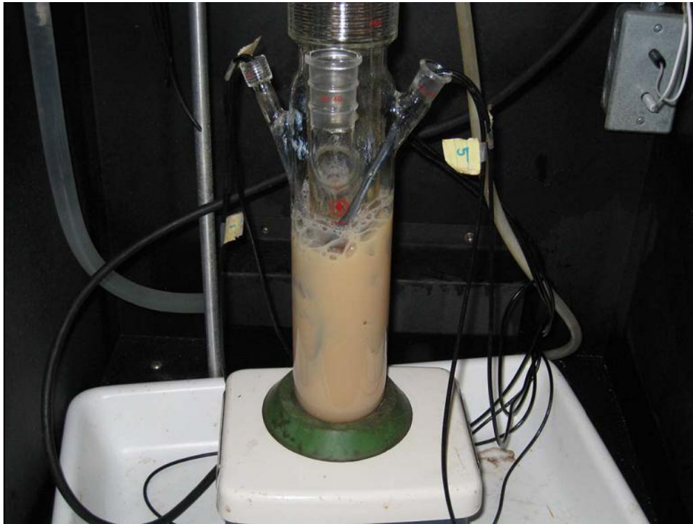
Figure 21: Experiment #5 using a COD (KHP) synthetic leachate with \text{TiO}_2 particles (Degussa P25) at time, t = 1.0 hour
