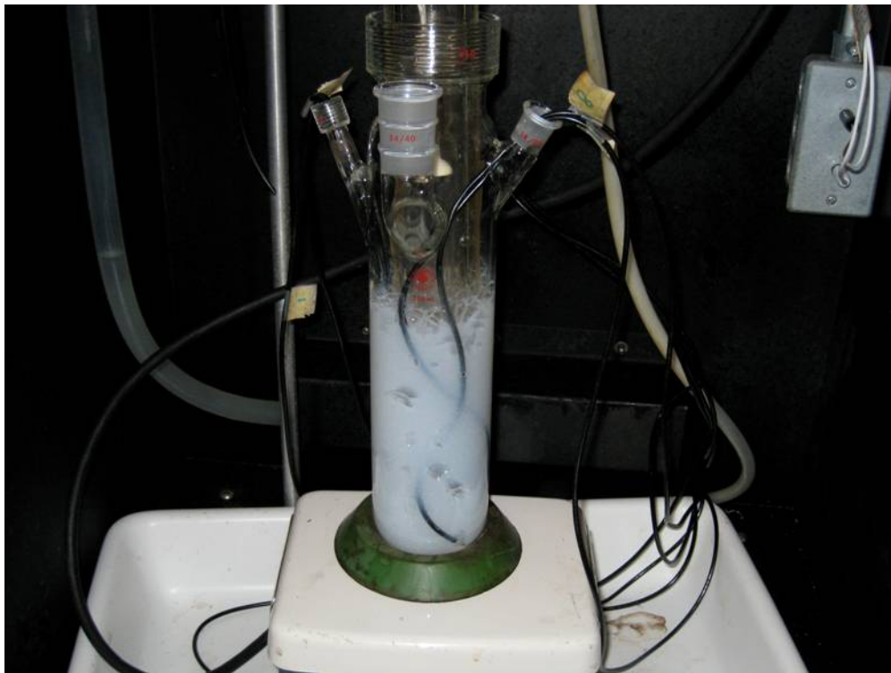
Figure 20: Experiment #5 using a COD (KHP) synthetic leachate with \text{TiO}_2 particles (Degussa P25) at time, t = 0 hours
