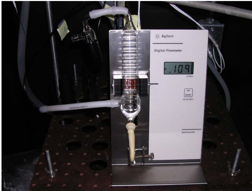
Figure 18: Measurement of the air flow rate.
