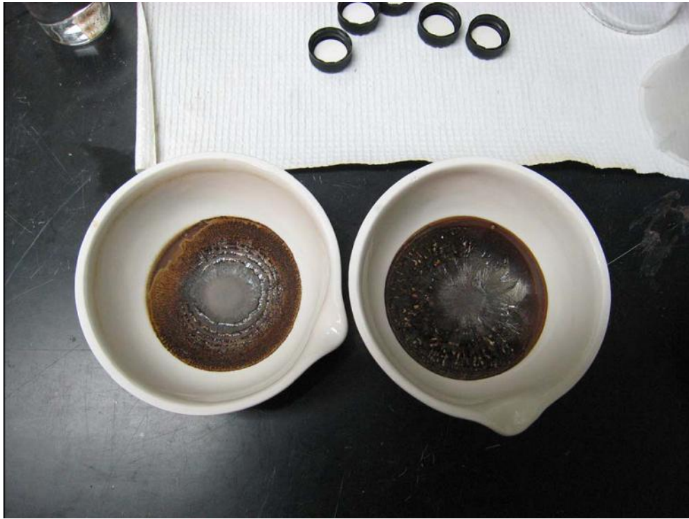
Figure 23: Experiment #5: Reconditioning (drying at 105°C for 24 hours) of left over TiO 2 particles after treatment of synthetic leachate containing COD
