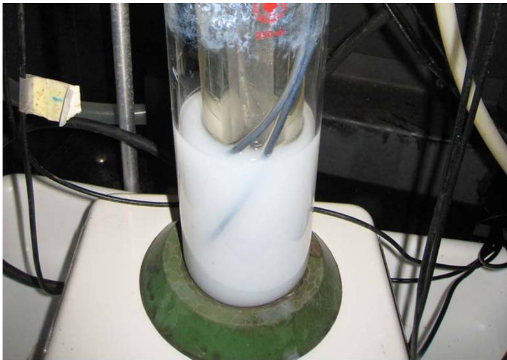
Figure 21: Experiment #5 using a COD (KHP) synthetic leachate with \text{TiO}_2 particles (Degussa P25) at time, t = 1.0 hour
