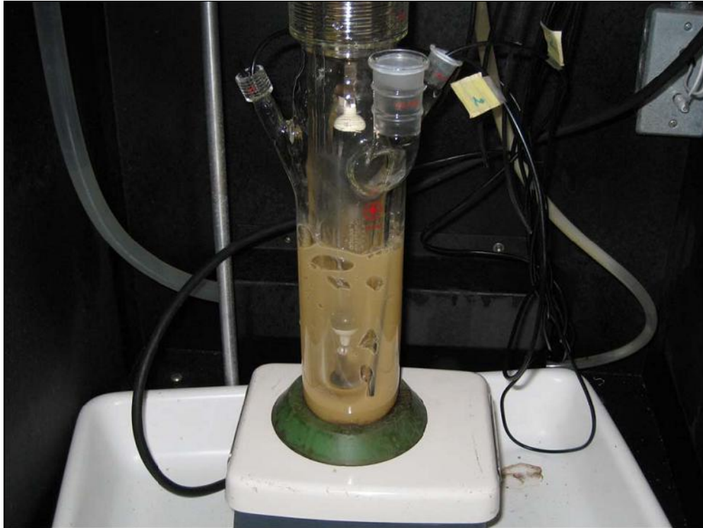
Figure 19: Experiment #2 using an ammonia leachate with \text{TiO}_2 -magnetite particles
