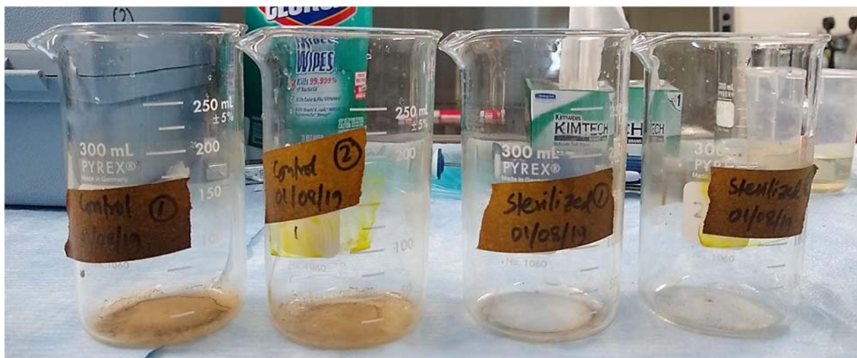
Figure 4. Visible adherent scale formation in 250 mL beaker for control (1st and 2nd from left) and sterilized sample (3rd and 4th from left)
