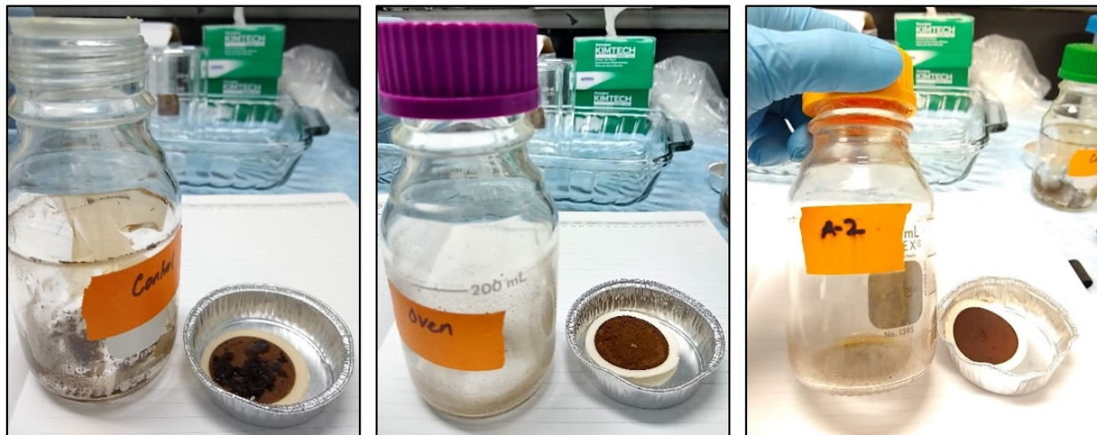
Figure 10. precipitate in the vessel surface and 4.5-micron filters for control, oven sterilized and Autoclaved leachate sample from left to right respectively
