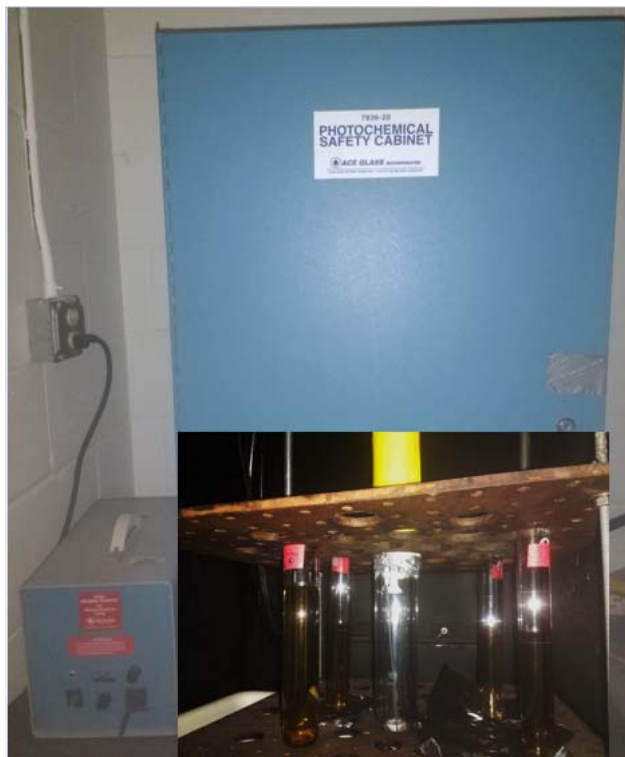
Figure 1. Photocatalytic Safety Cabinet used to disinfect leachate in the laboratory
