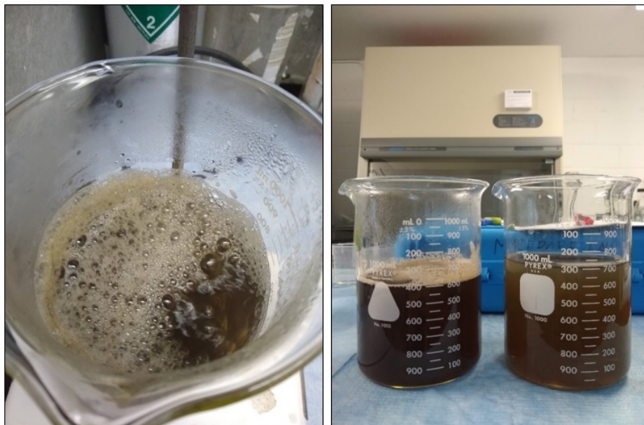
Figure 3. Boiling leachate (left), and visual comparison of sterilized and control leachate (right)
